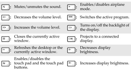
**Note:** If you changed the **HotKey Mode** from **Enabled** to **Disabled** in the BIOS setup utility, you will need to press the Fn key in combination with the appropriate hotkey.
